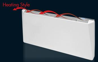
SIRIO will heat your home using natural convection - the cold air passes through the lower grille, is heated by the aluminium coil, and comes out of the grille at the top, heating your domestic environments perfectly, in complete safety and without any noise, as there are no moving mechanical parts.
